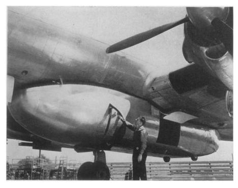
HEAVY LOAD—With a loaded Speedpak firmly attached to its fuselage, a Lockheed Constellation is given final check by a mechanic prior to flight. Water-tight sealing on the joint between the Speedpak and the Constellation fuselage prevents seepage of moisture in flight. A waterproof tarpaulin gives additional protection for the baggage compartment.
