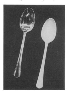
ONE OPERATION—The teaspoon on the right has been silver plated but not polished. The other has undergone the new-born electro-polishing process perfected by a physicist in the Westinghouse Research Laboratories. The new method may supersede the burnishing of silver plate by mechanical buffing. The transformation takes a little more than a minute.
