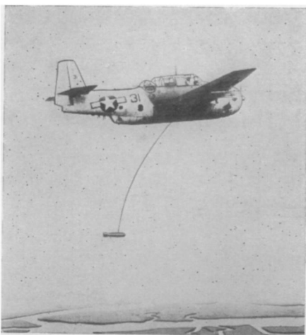
MAGIC EYE —Here we see the magnetic detector being flown from the wing of a plane as it will be used to locate oil below the surface of the continental shelves.
