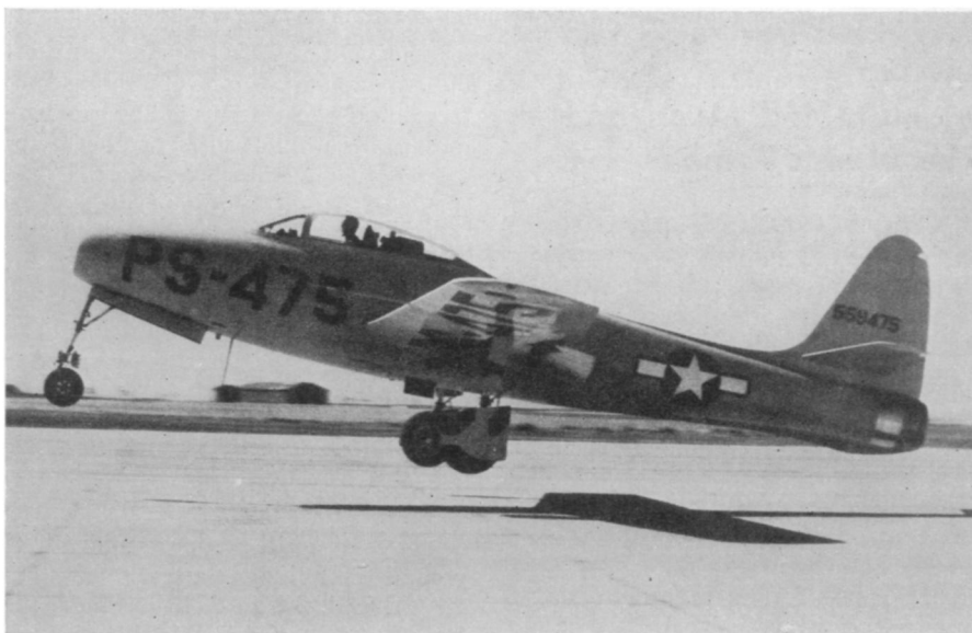
RECORD BREAKER —The Republic Thunderjet, new XP-84 jet fighter, has just been revealed by the army. Its speed is more than 590 miles per hour, and it has a service range of 1,000 miles and ceiling above 40,000 feet.
