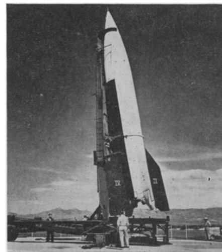
RESEARCH MISSILE—V-2 rockets have been fired higher than 100 miles into the stratosphere. Special instruments replace TNT in the warhead and may be lowered by parachute after ejection. These instruments furnish data for scientists.
