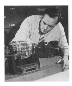
INSIDE LOOK—Transparent plastic model of an actual machine bearing shows the technic developed by a Westinghouse research engineer who needed to know what happened to lubricating oil inside a moving bearing. Oil, colored red, is fed into the plastic bearing and the lubrication effectiveness immediately is apparent.
