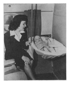
SKY CRADLE provides a seat and bed for baby airline passenger. Suspended by webbing on a tubular metal frame, the bassinet has a quilted plastic lining and wide belt fastened by a zipper across the child. Special waterproof lining for exclusive use is provided.
