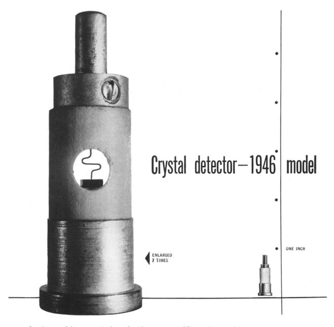
Remember the crystal detector in the first radios—hunting for the right spot with a cat's whisker? For years the detector lay discarded in favor of the vacuum tube. But when microwaves came, and with them the need to convert minute energy to amplifiable frequencies, a Bell Laboratories scientist thought back to the old crystal.
