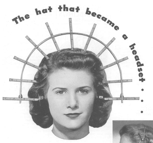
Telephone operators in New York, Atlanta and Montreal wore the strange head-dress you see pictured above. It's a specially devised gauging instrument — Bell Laboratories scientists used it to measure head contours in designing the new operator's headset.
