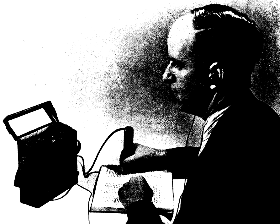
HEARING AID —Electronic device, developed in laboratories of the Radio Corporation of America, operates as a stylus on a printed page, translating letters into sounds.
