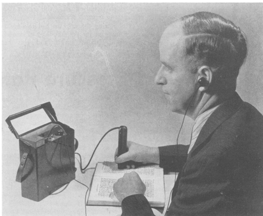
HEARING AID —Electronic device, developed in laboratories of the Radio Corporation of America, operates as a stylus on a printed page, translating letters into sounds.
