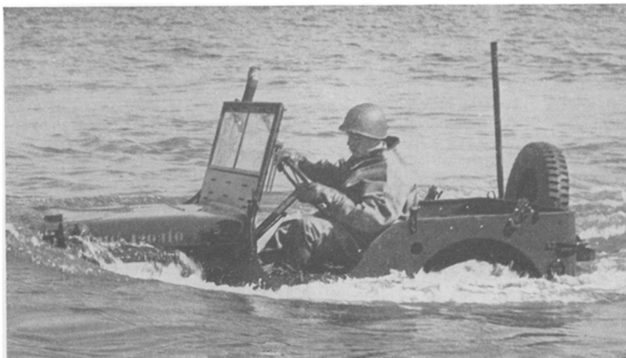
SUBMARINE JEEP —"Deep-water fording kits" equip jeeps for underwater operation at beaches and in fording streams. The jeep is made operable in water one foot higher than the hood for a period of 15 minutes. (See SNL, Oct. 26.) Official U. S. Navy Photograph.
