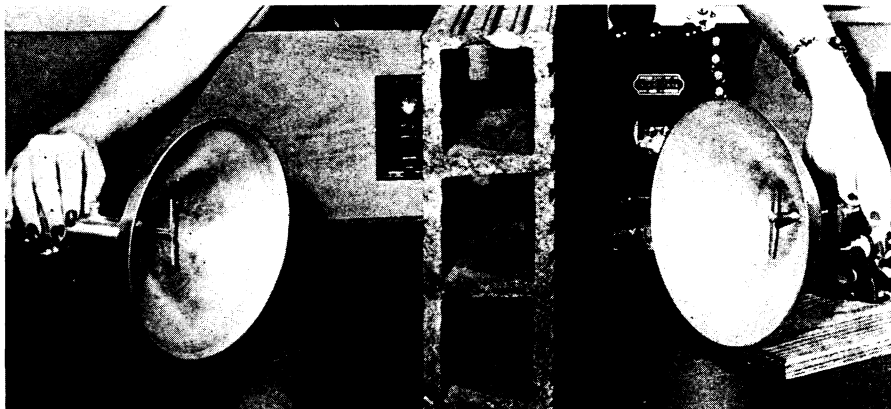
SEEING THROUGH TILE —"Microwave units," General Electric devices, use high-frequency radio waves to "see" through or around solid walls.
