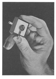
in radio receivers. This selenium rectifier, of the metal plate type, can be used to charge a two-volt battery in a battery portable set, and also deformed electrolytic condensers.
