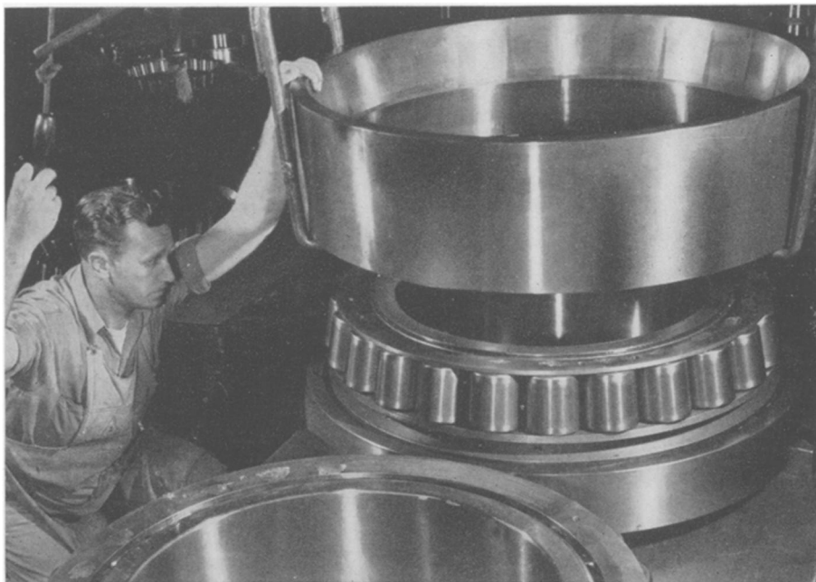
CROWNING IT —Outer ring is being put on enormous tapered bearing.
