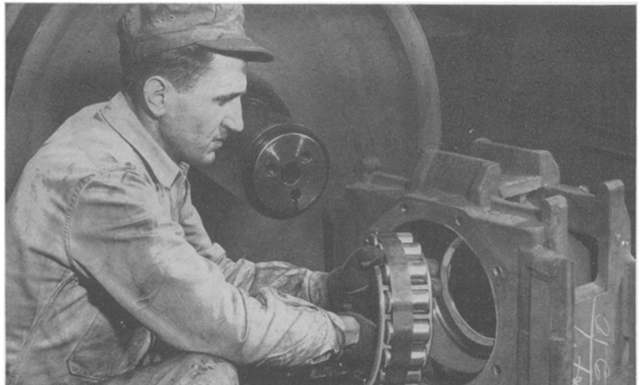
LUBRICATION —Eliminating hot-boxes, roller bearings installed on high-speed locomotives and trains are lubricated only when the equipment is brought into the shop for general inspection. Ball and Roller Bearing Information Center photographs.
