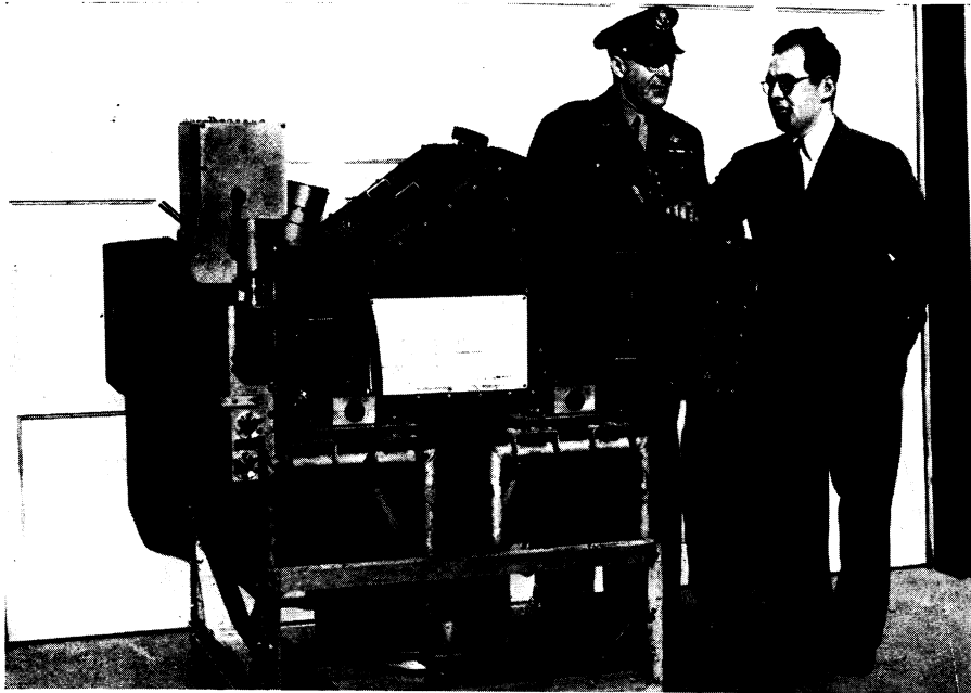
AERIAL PHOTOGRAPHY —The giant 200-inch lens camera developed by the Army Air Forces at Wright Field takes pictures from 30,000 feet in the air.
