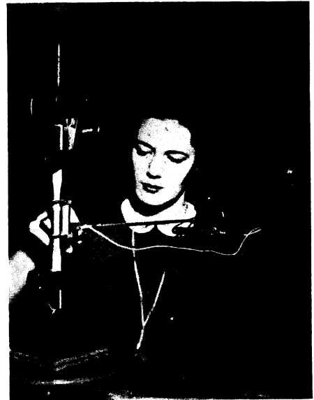
STRENGTH TEST —The tensile strength of a plastic specimen is measured at the National Bureau of Standards. The sample's elongation under tensile force, applied by a universal testing machine, is measured by an extensometer and recorded automatically on a chart.
