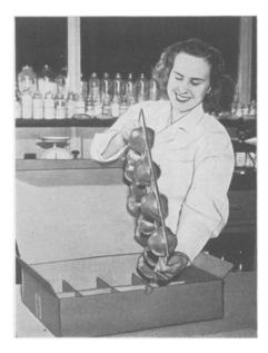
The film across the holes, when heated slightly, stretches to fit the fruit, shown in the picture.
