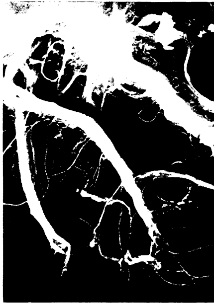
TINY FIBRILS —Ground wood pulp structure revealed under an electron microscope.
