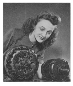
MODERN MOTOR for shop or home, one-quarter horsepower capacity, is about one-third the size and weight of its 43-year-old ancestor. The enclosed housing of the new motor, as can be seen from the picture, protects the rotary parts from dust and grit.
