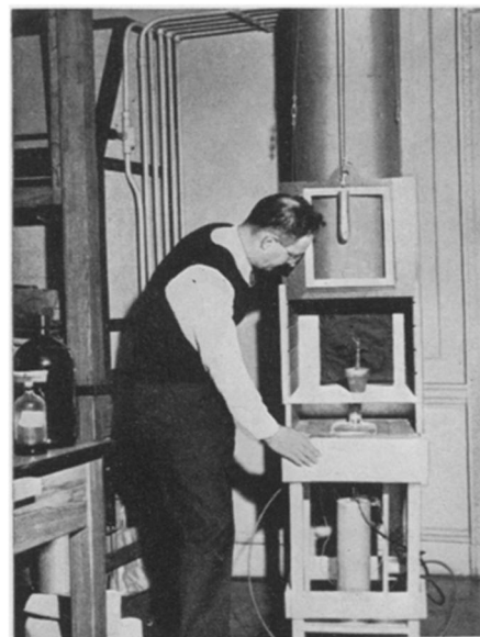
TESTING TOWER —Duster, tower, and dust distributor are shown in this photograph from the Pennsylvania Salt Manufacturing Company.
