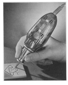
ELECTRIC TOOL for woodworkers and others has 36 interchangeable accessories such as abrasive wheels, drills, buffing wheels and brushes. Housed in a shockproof plastic case with an aluminum frame, the motor shaft extends to a metallic tool-gripping nose as shown in the picture.
