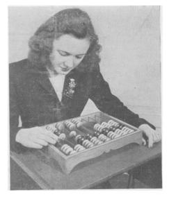
multiplying and dividing. The fifth and sixth digit disks on each rod, as shown in the picture, are larger than others to speed operation and particularly to assist the blind.
