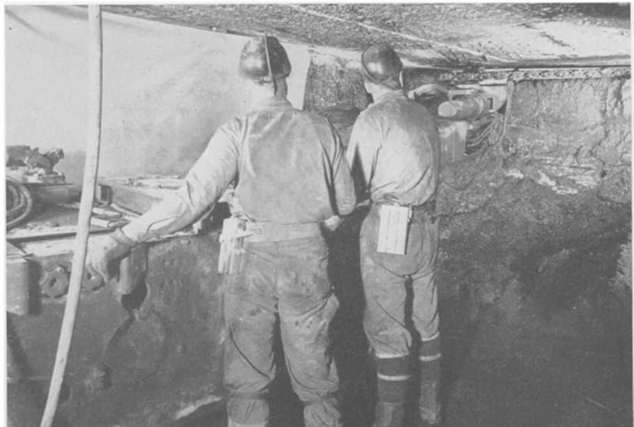
MECHANIZED MINING —American coal miners use machinery electrically operated such as the machine cutter shown in the picture. Loosened electrical connections, or sparking caused by dust collection in the machine may cause explosions.
