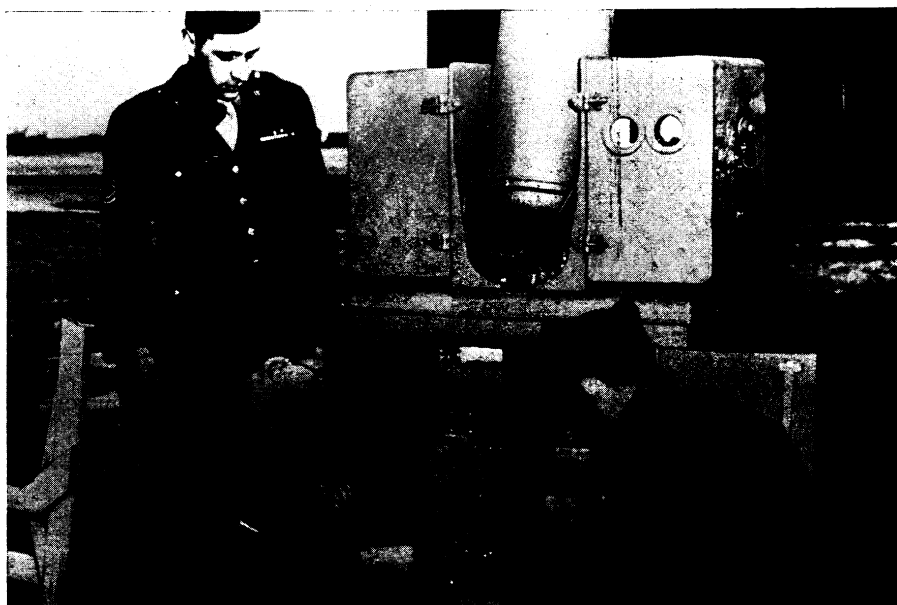
CEILOMETER —Army Air Forces instrument measures the height of clouds by throwing up a ray of ultraviolet light which is scanned by a photo-electric cell unit. When a cloud breaks the beam, a "trace" registers on the recording instrument. The ceilometer accurately gauges cloud heights up to 10,000 feet.
