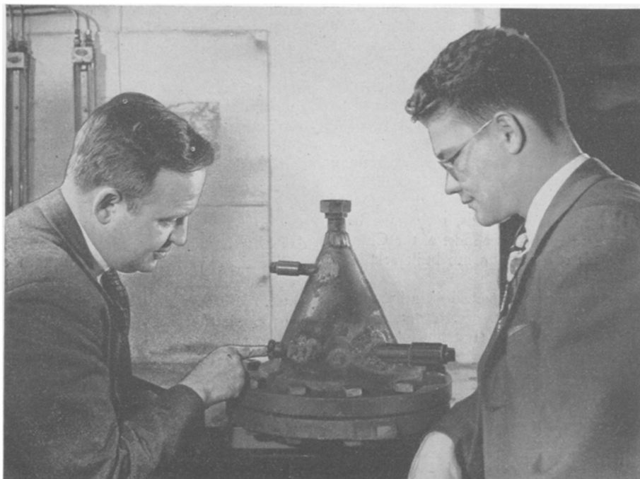
FLOWING COAL —"Coal atomizer" and attrition chamber are being examined by John I. Yellott, director of research, and W. N. McDaniel of the Locomotive Development Committee of Bituminous Coal Research Laboratory at Johns Hopkins University
