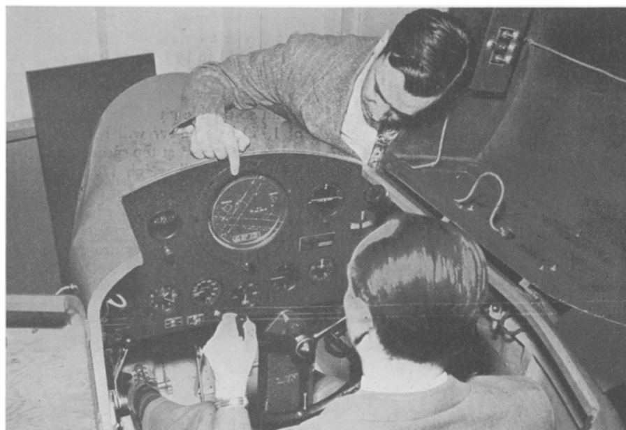
TELERAN —The new RCA television-radar air navigation and traffic control is installed in the cockpit of a flight simulator. Data are shown on a screen on the instrument panel.
