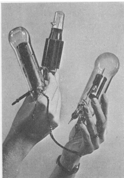
COUNTER TUBES —Each of these, used in Geiger counters, has a different ray-detecting job.
