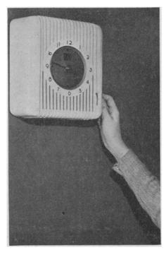
RADIO-CLOCK combination is housed in an attractive plastic casing arranged either to stand on a table or hang on a wall. The electric clock, placed in the center of the case, as shown in the picture, cleverly conceals the radio.
