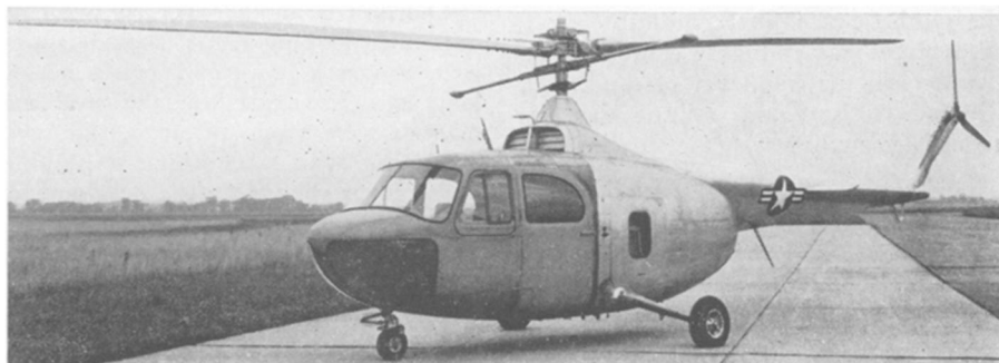
FIVE-PLACE HELICOPTER —The Army XR-12, with a top speed of 105 miles an hour, is undergoing preliminary tests. A two-bladed rotor system is used with a gyroscopic action stabilizer bar.
