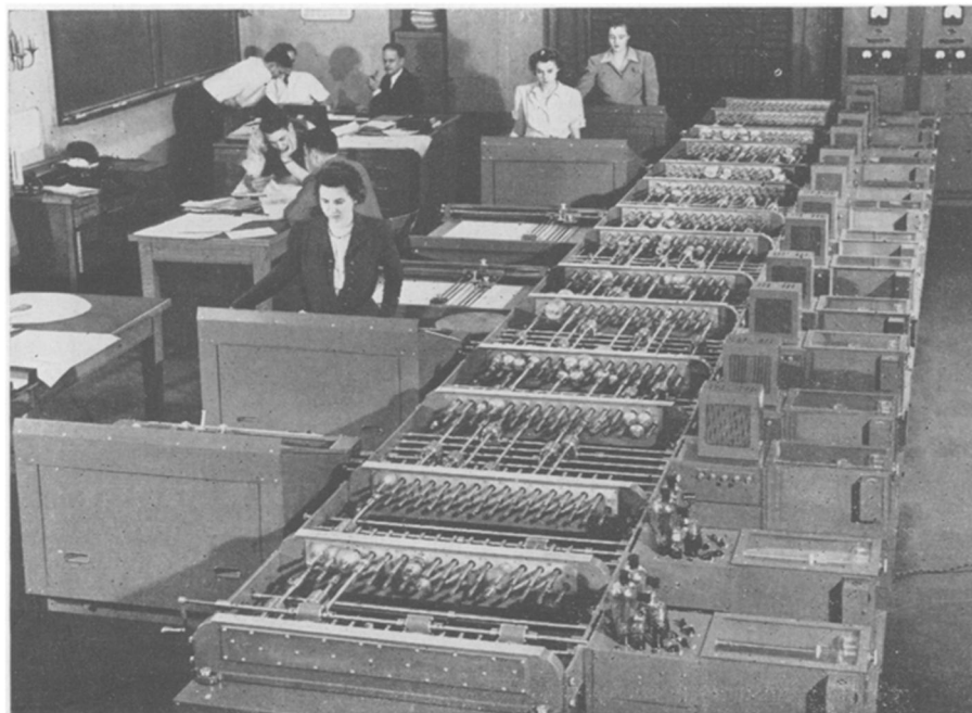
MATH BY MACHINE —This differential analyzer has accomplished in two weeks computations equal to 17 man-years of effort. Although the machine operates mechanically, it is electrically controlled. It has become part of the "figure center" at U. C. L. A.
