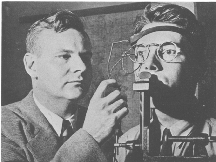
ELECTRIC RESPONSE —Dr. Lorrin A. Riggs, psychologist at Brown University, measures the electric current on the eye of his co-worker, E. Parker Johnson, by means of an electrode inserted in a contact lens. In this way it is possible to measure the eye's visual sensitivity. (See SNL, Nov. 29.)
