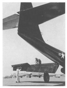
AIR BRAKES—The jaw-like control surfaces shown above at the outer end of the wing trailing edge on a Northrop Scorpion, twin-engine, jet-propelled, all-weather fighting airplane are known as "decelerons" because they combine the functions of ailerons, fighter brakes and landing flaps. In normal flight the jaws are closed. In dives, the jaws are opened to provide effective fighter brakes.
