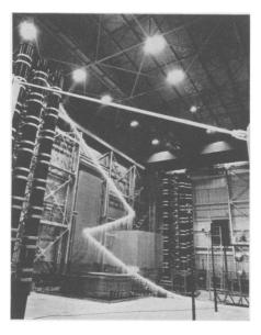
MAN-MADE LIGHTNING — A streak of flame, then complete vaporization is the fate of a strand of copper wire charged with 5,000,000 volts of electric power in the new GE High Voltage Laboratory.
