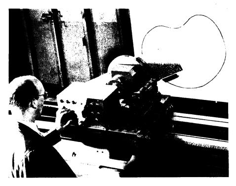
ELECTRONIC CUTOUT—Called the "G-E contour following system," this instrument has an electric eye which follows the lines of a drawing through a microscope. It is connected to a metal-cutting tool which reproduces the drawing's outlines in metal. Developed by General Electric engineers, the device is designed to simplify manufacture of irregularly-shaped metal parts.
