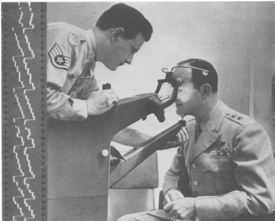
FASTER READING —First step is a film record made of the eyes with the ophthalmograph in the Pentagon's Reading Improvement Laboratory. Maj-Gen. Kenneth P. McNaughton's eyes are photographed by the instrument, as it is adjusted by Staff Sergeant Thomas J. Smith. Film record (left) made by the ophthalmograph reveals the number of stops or fixations made by the eyes in reading lines of type.
