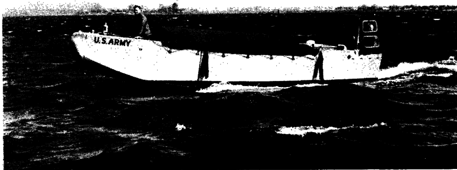
SECTIONAL CARGO BOAT —Built in three parts, and easily disassembled, this 32-foot, all-aluminum, Army cargo boat was designed so that it can be transported in a cargo plane, and is intended especially for Arctic operations. The rear section, with its 60-horsepower engine, can be used as a separate power unit to propel rafts and barges.
