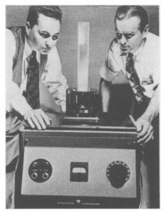
SILENT SOUND GENERATOR—Quartz crystal, contained in the translucent plastic case on top of the cabinet, generates high frequency sound waves pitched so high that the human ear cannot hear them. The new generator was developed by General Electric for research into the possibilities of putting the inaudible waves to work.
