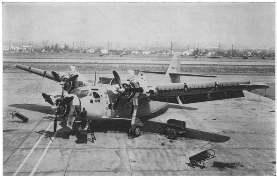
ASSAULT TRANSPORT —The Northrop Raider C-125 has been designed to make all parts of the plane easily accessible for repairs.
