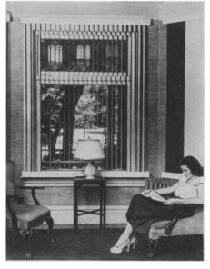
concealed control rod opens or closes the louver to any degree, and each of these fabric parts may be removed for cleaning by slipping it from tiny hooks at the bottom and top.
