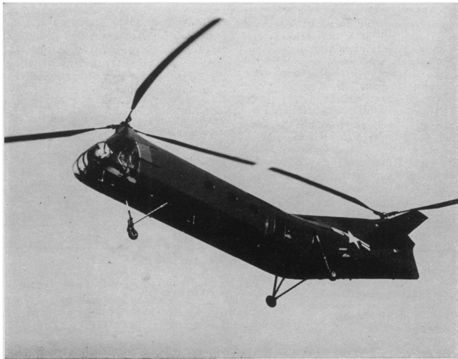
STREAMLINED "FLYING BANANA" —The Navy's new Piasecki HRP-2 is pictured during early flights at Morton, Pa. Its aluminum fuselage is the latest development in helicopters in the program to help America maintain leadership in transport type rotary wing aircraft. As many as 12 litter patients can be carried in the HRP-2. This type of aircraft is particularly suitable for mass rescues under the most adverse conditions and for troop-carrying assault tactics.
