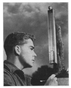
graduated tube, easily read, can be removed from the metal holding frame for emptying.
