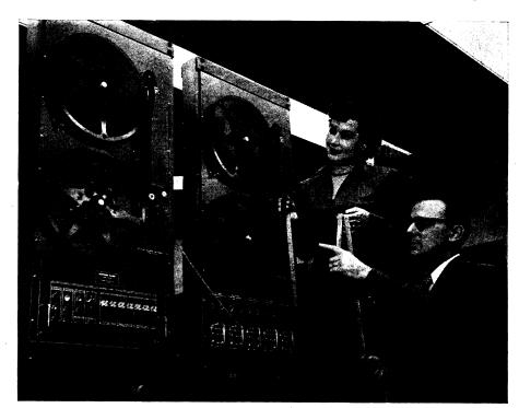
AIRPORT RECORDER—The ingenious machine makes possible for the first time a permanent record of all communications between pilots and control towers, thus permitting a detailed study of factors leading to air crashes. Hailed as a great advance in aviation safety, it records up to 28 voices on a single magnetic paper tape less than three-quarters of an inch wide.
