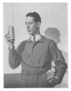
code signals, and has a pick-up range of 80 miles. Instrument and battery are unaffected by salt water.
