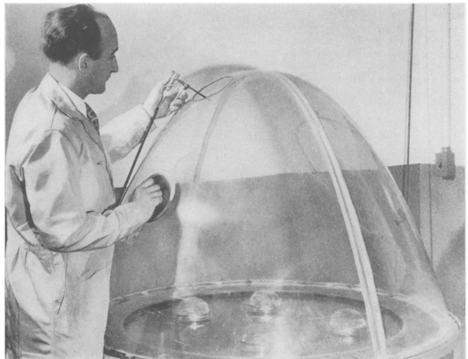
BLISTER TEST —The effect of allyl cinerin, a pyrethrum insecticide, is tested on cockroaches (under small screens) by Dr. Harry L. Haynes, entomologist at Boyce-Thompson Institute. Though not an official test method, this "blister" is a means of observing the effect of the insecticide with non-clogging and non-staining properties not possessed by the natural product.
