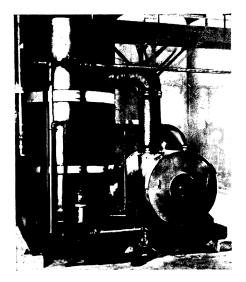
OUT WITH THE BRINE—Heat distills sea water making it pure enough to drink. The compression distillator, made by the Arthur D. Little Company, Cambridge, Mass., allows the reuse of the original heat, thus cutting down fuel costs.
