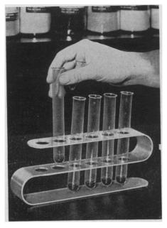
Shown in the picture, is a flat "S" in shape and is made of aluminum. This corrosionresistant metal rack is superior to the longused racks of wood because it is more durable and can be used in drying ovens.
