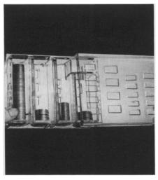
nickels and quarters. Coins are placed in the proper column and their total value noted by a calibrated scale beside the column.
