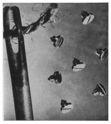
are said to be the world's smallest massproduced precision screws. They are used in precision watches and several types of military timing instruments.
