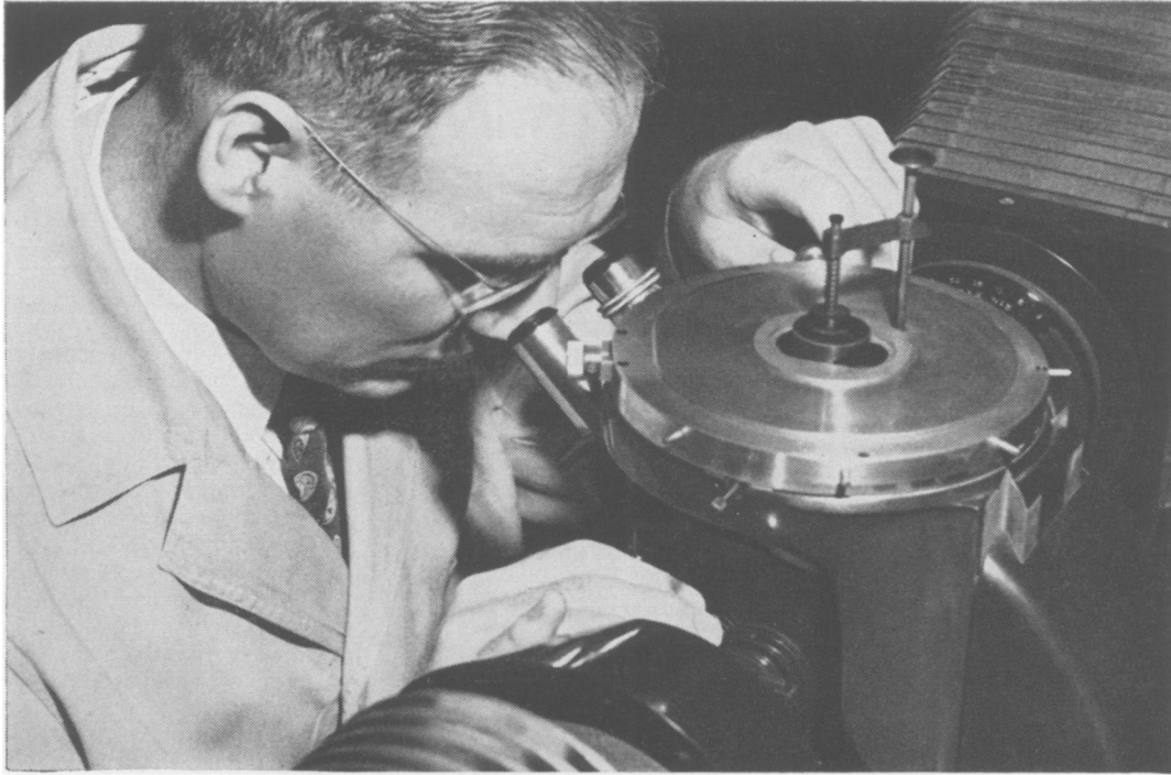
Examining specimen on metallographic microscope at Bell Telephone Laboratories
